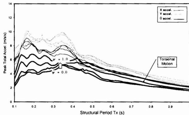
Figure 4: 95% spectral envelope for Soil Class 2
