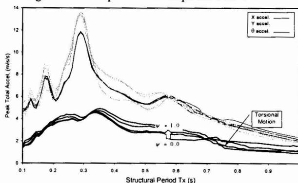
Figure 8: 95% Spectral envelope, Soil Class 1, Alaskan subduction Earthquake, 1964
