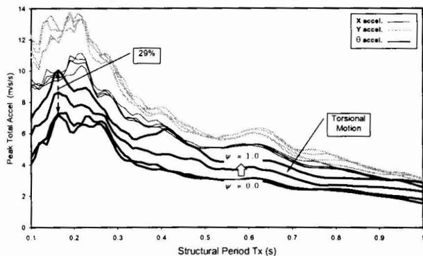
Figure 3: 95% spectral envelope for Soil Class 1
