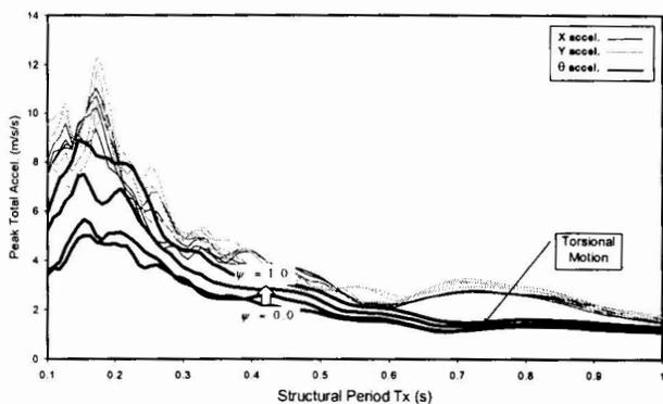
Figure 7: 95% Spectral envelope, Soil Class 1, Whittier Narrows Earthquake, 1987
